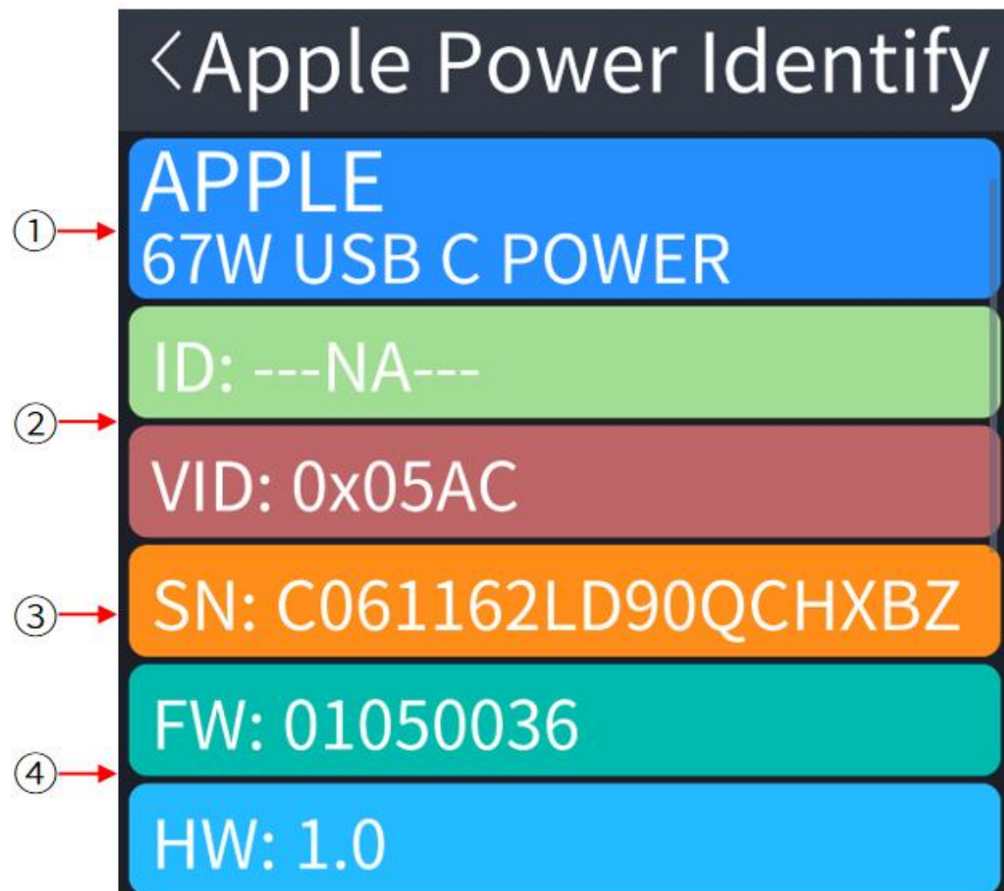
Figure 2.10 Apple Charger Identification Interface
